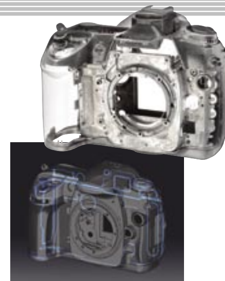
Principal points where sealing protects against drops of water and dust
